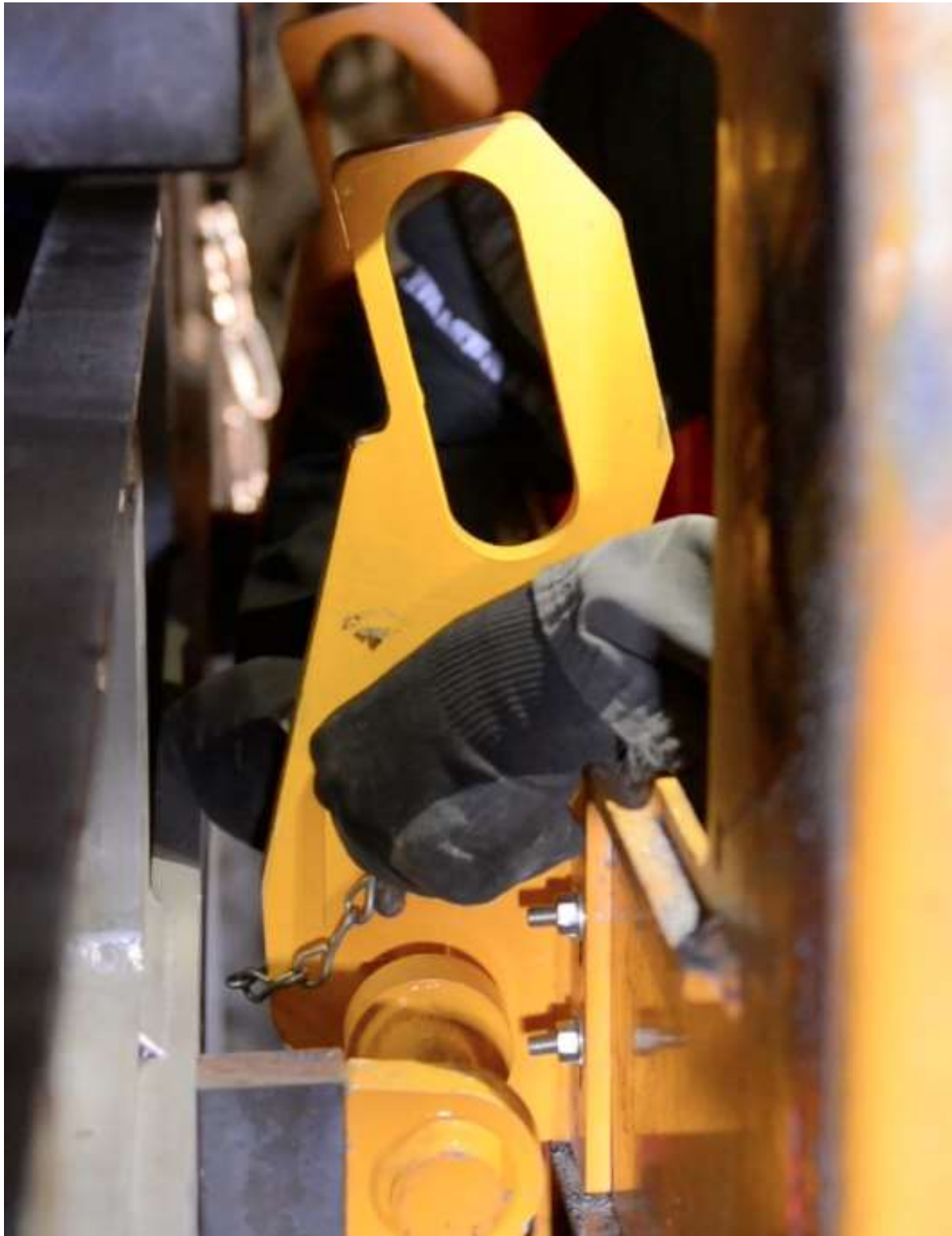
Figure 9 – The Locking Handles Securing the Basket to the Equipment
