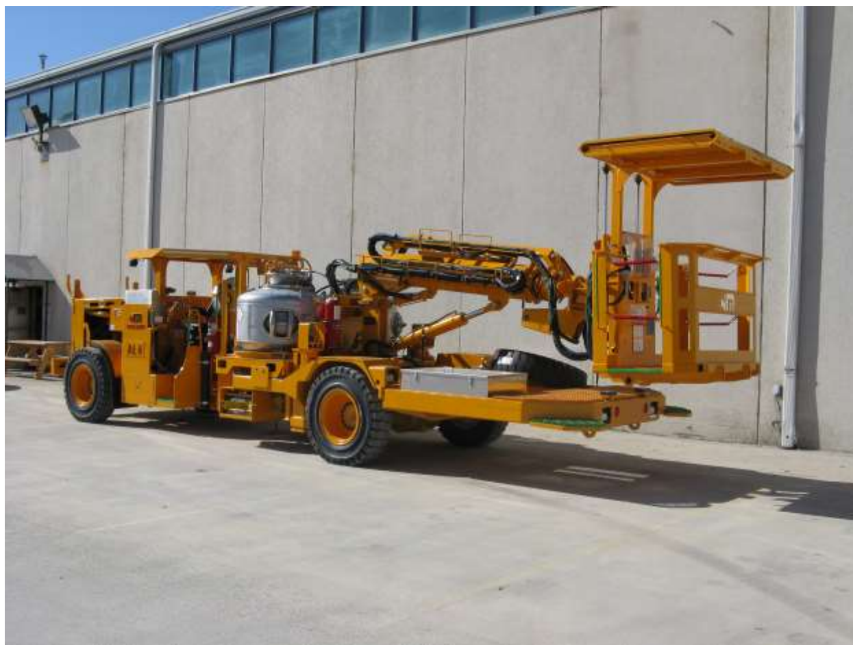
Figure 1: Mechanical Hood on a Basket
