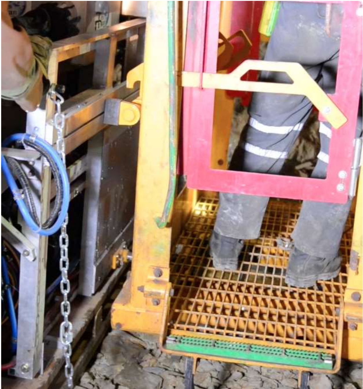
Figure 8 – The Face of the Basket in Position Against the Equipment Storage Pallet
